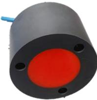
ETS50200 is the latest dual transducer from SKIPPER. It operates on 50 and 200 kHz frequency. SKIPPER has now made a special version in order to fit the old Elac Tank for retrofit. This will make a retrofit of the Elac system easier without any welding operation. You will need a diver or a dry-dock in order to do the retrofit.
